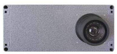
Traversing scanner with halogen lamp and spectrometer
